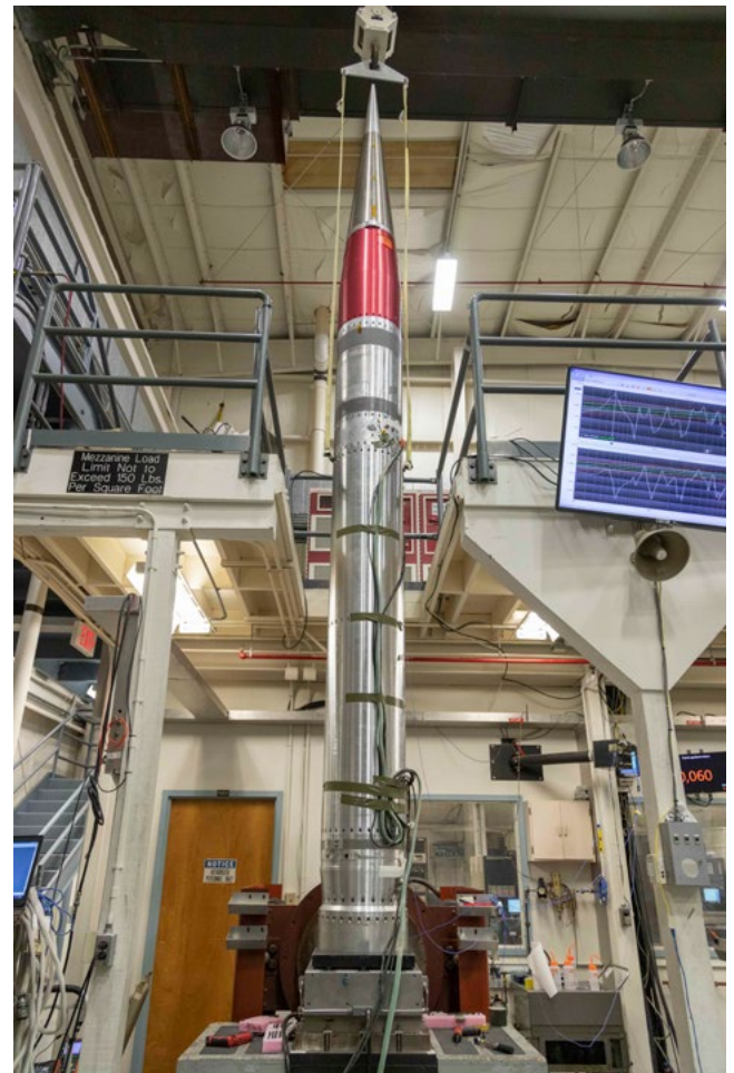
HOTShot payload on the vibration table at Wallops.
